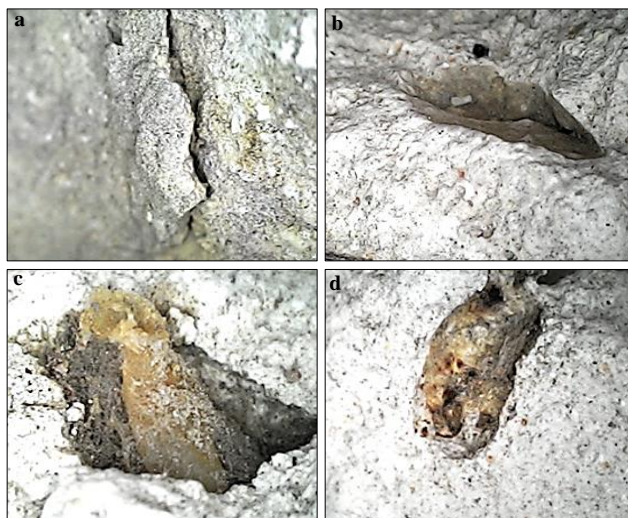
Figure (4) stereo light microscopy images, 40x; a. & b. macro and micro-cracks, c. & d. nests of wasps
