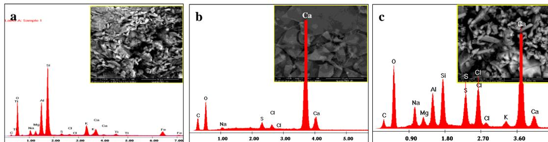
Figure (4) XRF patterns and SEM photomicrographs showing a. marly limestone b. shell stone, c. mortar
