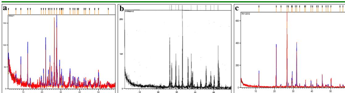
Figure (3) Some XRD pattern of different types of stone a. marly limestone, b., shell, c. mortar
