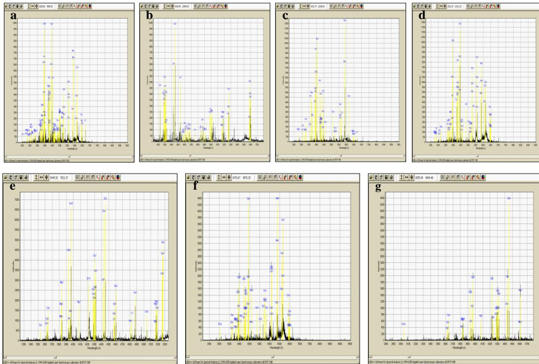
Figure (5) LIBS spectrum showing **a.** marly limestone **b.** sandy blood dolomite, **c.** artificial stone, **d.** phyllite, **e.** white marble, **f.** shell stone, **g.** mortar
