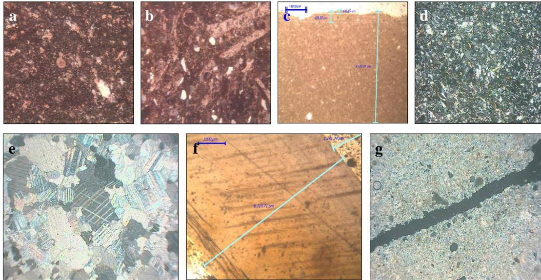
Figure (2) Thin section investigations showing **a.** marly limestone (quartz, feldspars & hematite), **b.** sandy blood dolomite (quartz, feldspars & calcite), **c.** artificial stone (different sizes of quartz), **d.** phyllite (quartz & feldspars), **e.** white marble (calcite), **f.** shell stone, **g.** mortar (quartz, lime & gypsum)
