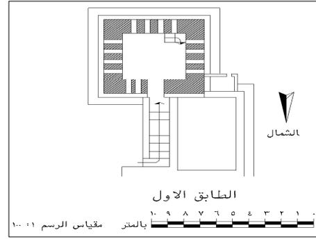
Figure (12) tabia plan of the 1<sup>st</sup> floor
