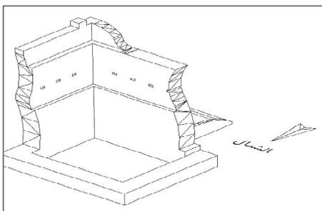
Figure (17) S. & W. walls of the ground and 1<sup>st</sup> floors
