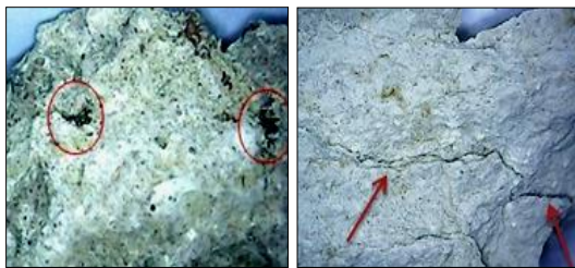
Figure (5) Shows DM photographs showing the caves and micro-cracks distributed in the surface of limestone samples
