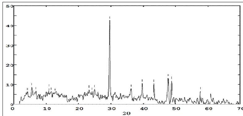
Figure (8) XRD pattern of plaster and colors as follow (Calcite  $\text{CaCO}_3$ ) (Hematite  $\text{Fe}_2\text{O}_3$ )
