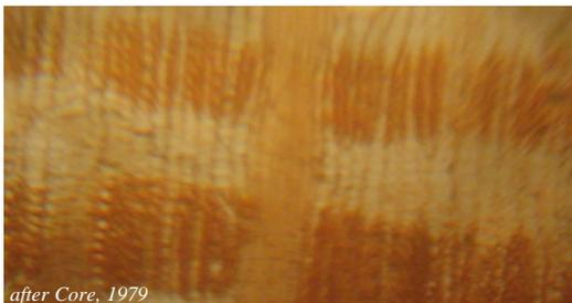
Figure (4) light microscope photo of (T.S) section confirming that the type of the wood is *Pinus sylvestris*
