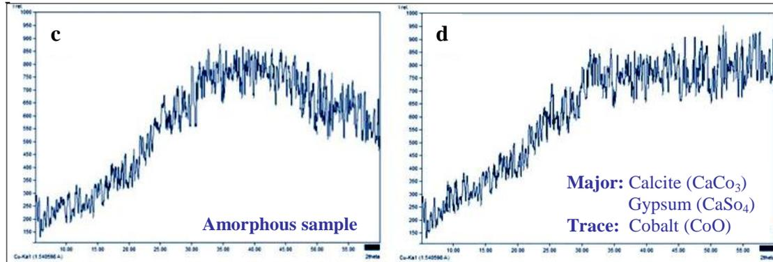
Figure (6) Shows XRD patterns **a.** a sample of blue glass, **b.** a sample of turquoise glass, **c.** a sample of green glass, **d.** a sample of dark brown glass.
