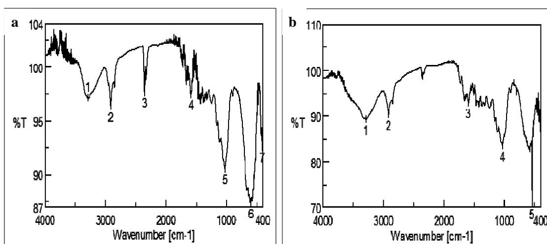
Figure (6) Shows FTIR chart of **a**, the wood fibers sample, **b**, deteriorated parts sample
