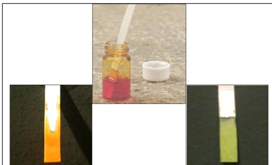
Fig. (1) Shows change of the checker color due to the PH value
