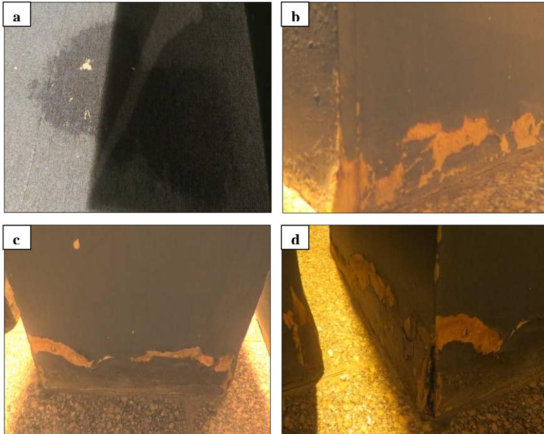
Figure (9) Shows deteriorated forms **a**, wet carpets, **b**, **c**, **d**, wooden bases under the artifacts
