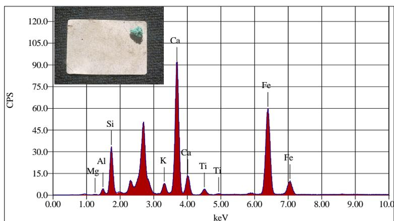
Fig (7) Shows XFR chart of little airborne dust sample collected present over the strips
