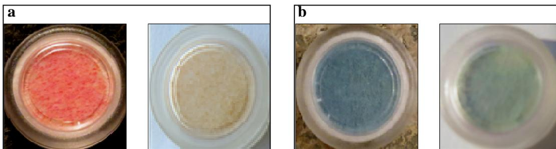
Fig (2) Shows the pamphlet of the passive indicator interference gas **a**. Ammonia gas detector, **b**. Organic acids detector
