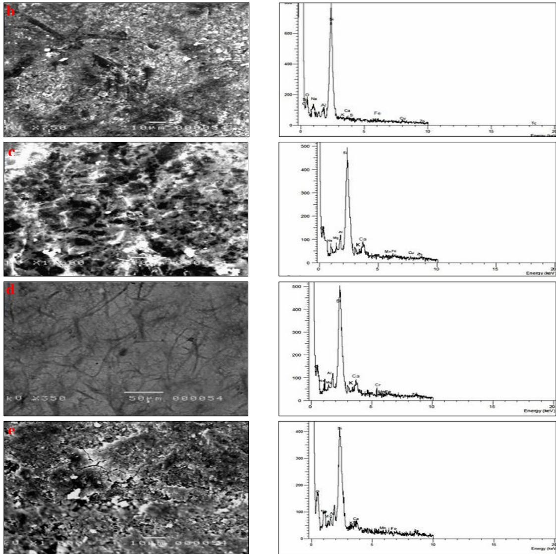
Figure. (6) Shows SEM photo-microphotograph and EDX charts **a.** a sample of blue glass, **b.** a sample of brown glass, **c.** a sample of red glass, **d.** a sample of green glass, **e.** a sample of dark brown glass with black tracing line
