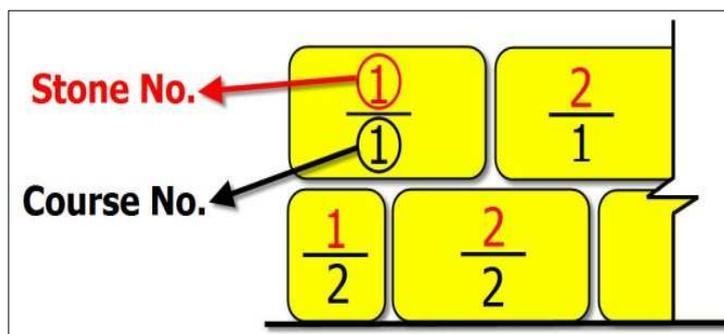
Figure (9) Shows method of stones punctuation of Dedan wall
