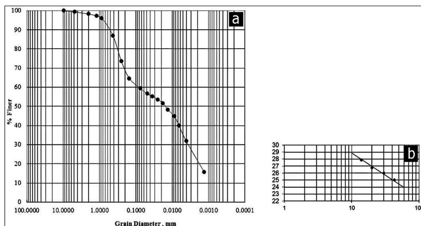
Figure (8) Shows **a.** grain size distribution curve for Dedan site, **b.** determination of Atterberg limits of soil
