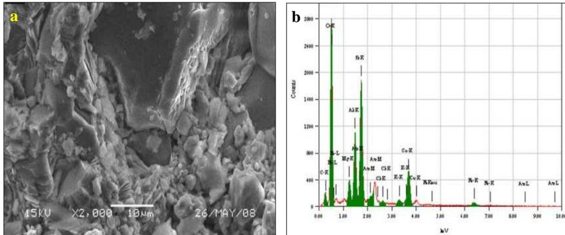
Figure (7) Shows **a**. the deformation of quartz, **b**. EDS analysis of red sandstone
