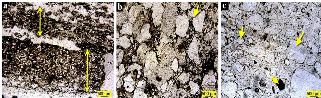
Figure (5) Shows **a.** laminated yellow sandstone, **b.** red sandstone, **c.** gray to white sandstone
