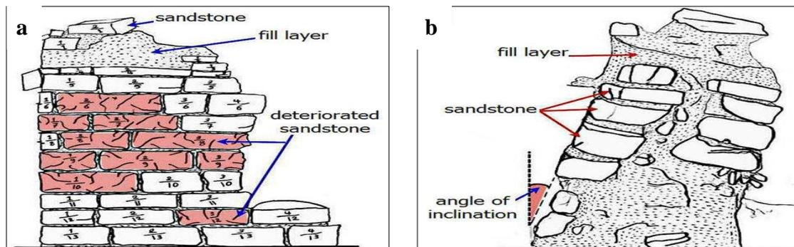
Figure (11) Shows **a.** identify deteriorated stones in the eastern direction, **b.** detailed drawing shows the stone wall condition from the northern direction
