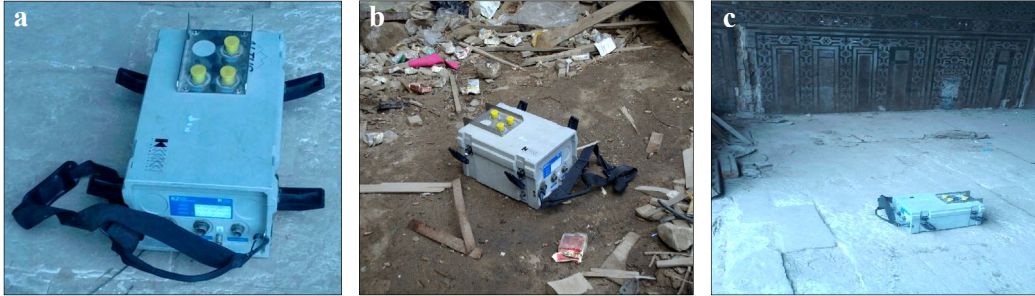
Figure (4) a. K2 Altus accelerograph used to record the ambient noise of the present work, b. recording at the soil in front of Mekaad Radwan, c. recording at first level of Mekaad Radwan
