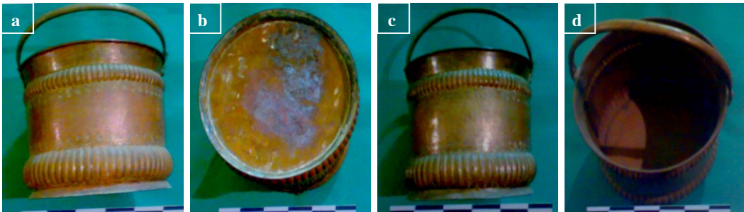
Figure (2) a Two water bucket before cleaning, b bottom of 1 st water bucket containing a lot of green corrosion compounds, c the water bucket before cleaning, d different corrosion products inside the second water bucket
