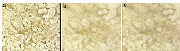
Figure (4) surfaces' appearance; a. un-treated, and the approx. same point of the sample, b. after treatment, c. after aging.
