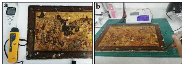
Figure (6) measurement of a , moisture condition, b , pH value.
