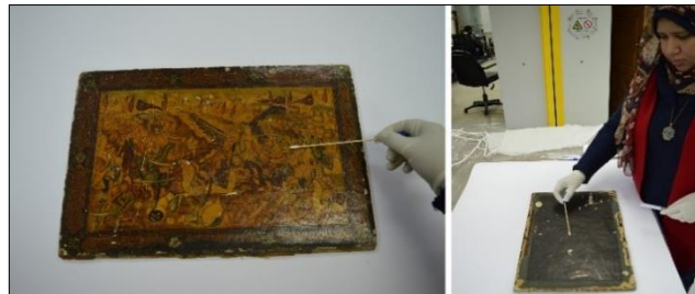
Figure (2) the method used to collect a sample of biological swab in order to identify the presence of biological damage.
