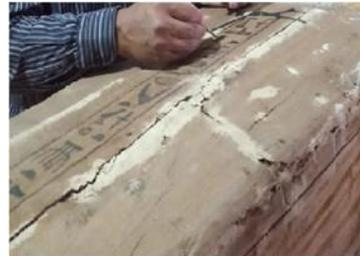
**Figure (11)** isolated the inscriptions and colored scenes on the coffin lid and coffin, in order to preserve from damage during the subsequent conservation processes, by using Klucel G (hydroxyl propyl cellulose).
