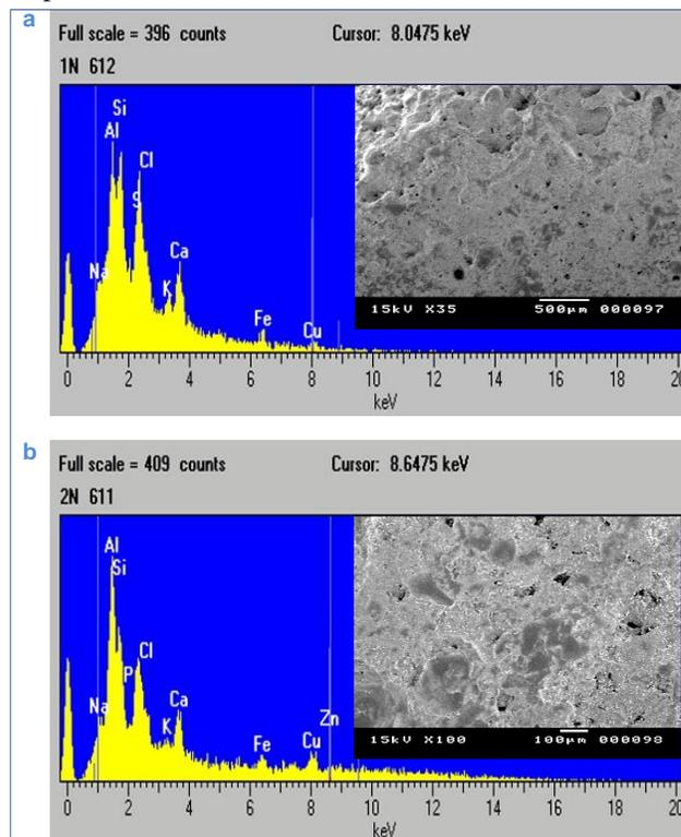
**Figure (6)** SEM photomicrographs & EDX patterns of the surface one of the faience beads **a.** sample 1, **b.** sample 2
