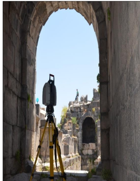
Figure (2) Laser scanner used for collecting 3D clouds of the monuments
