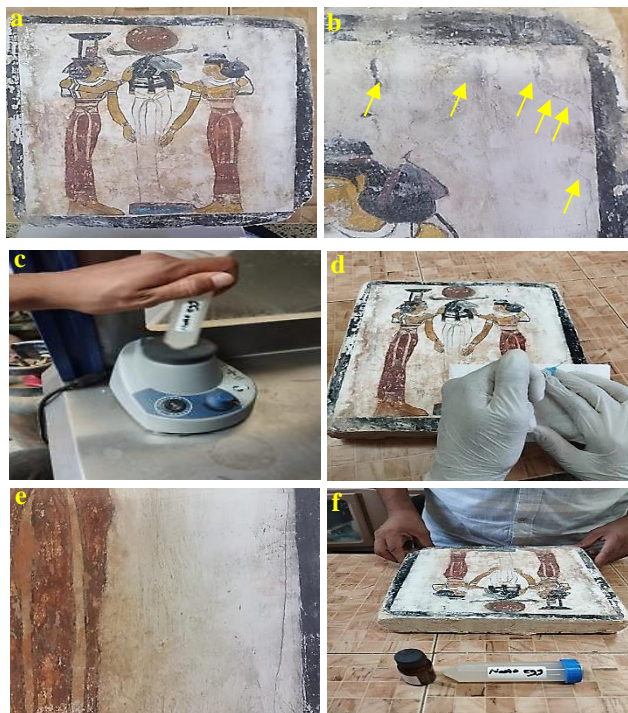
Figure 10 a. Experimental samples prepared with the same characteristics as the mural paintings in the tomb of Qen-Amun (TT93), b. horizontal and vertical cracks before, c. preparation of the eggshell nanoparticles by vortex and ultrasonic, d. cracks injection, e. Cracks after treatment, f. treated sample
