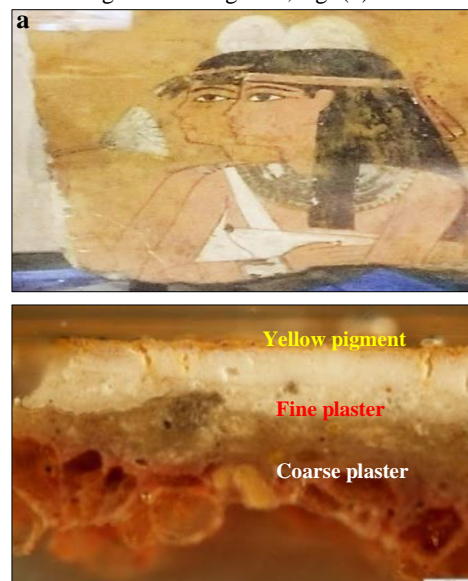
Figure (4) a , fragment of wall decoration, painted with depiction of two women, tomb of Qen-Amun (TT93), it was returned to Egypt as a gift from the clos foundation, Spain, on 30/1/2009 Luxor, b , cross-section image of the fragment with three layers from top to bottom (yellow pigment, fine plaster, coarse plaster) under PLM
