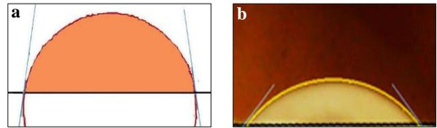
Figure (6) contact angle of **a.** new sample ( $70^\circ$ ), **b.** arch. bone sample ( $44^\circ$ ).
