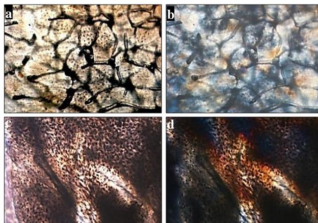
**Figure (4)** PLM of new and archaeological bone samples; **a., b.** new sample under plain light (100-X) and polarized light (100-X) respectively; **c., d.** archaeological sample under plain light (100-X) and polarized light (100-X) respectively.
