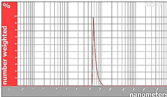
Figure (1) Shows NICOMP DLS curve of synthesized CNC
