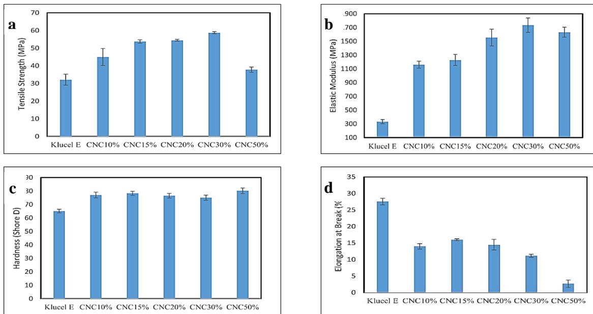
Figure (4) Shows mechanical properties of Klucel E/CNC nanocomposite
