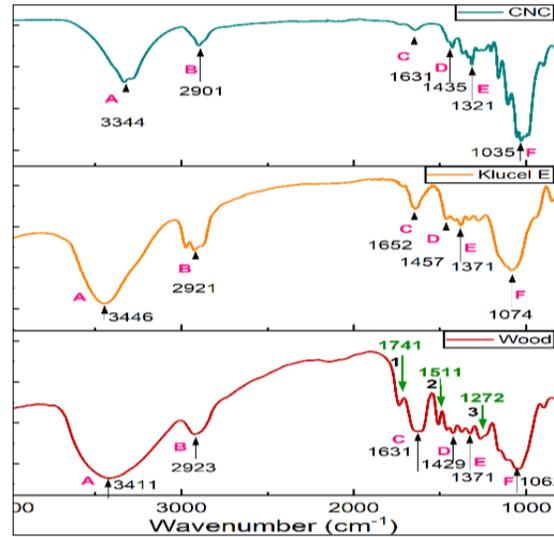
Figure (8) Shows FTIR spectra CNC, Klucel E and wood
