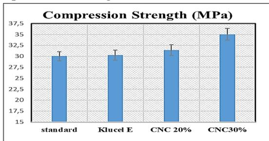
Figure (10) Compression strength for wood specimens consolidated with Klucel E, composites with CNC 20 and 30%
