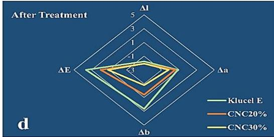
Figure (7) Shows comparison of color parameters of treated wood samples before and after aging: **a.** Klucel E, **b.** nanocomposite with CNC 20%, **c.** nanocomposite with CNC 30%, **d.** all materials after all impregnation process.
