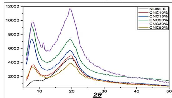
Figure (3) Shows XRD patterns of pure Klucel E, CNC 10%, 15%, 20%, 30% and 50%.
