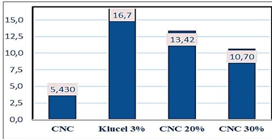
Figure (5) Shows viscosity measurements for CNC suspension, Klucel E 3% and CNC composites with 20% and 30%
