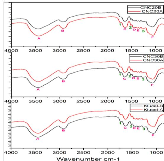
Figure (9) Shows FTIR spectra for consolidated specimens with composites CNC 20%, CNC 30% and pure Klucel E (black line = before aging & red line = after aging)
