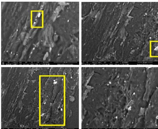
Figure (5) Shows SEM photomicrographs of a sample from one of the wax figurines, in good mixing and interconnected texture between wax and resins, the yellow rectangles indicate the presence of silica, as one of the materials used in the inner packing of the mummy which the wax statue was extracted.
