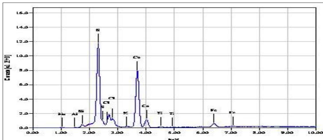
Figure (16) EDX patterns of analysis of the wood sample.
