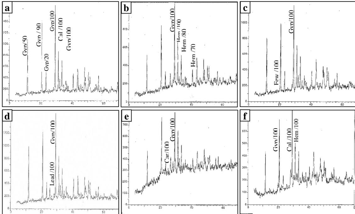
Figure (11) XRD pattern of the paint layers of Qaitbay's madrasa ceiling **a** white pigment **b** red pigment **c** blue pigment **d** brown pigment **e** black pigment **f** gilded layer.
