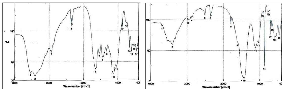
Figure (13) FTIR spectra showing, **a** FTIR sample of red pigment (animal glue) **b** FTIR sample of gilded layer (animal glue)
