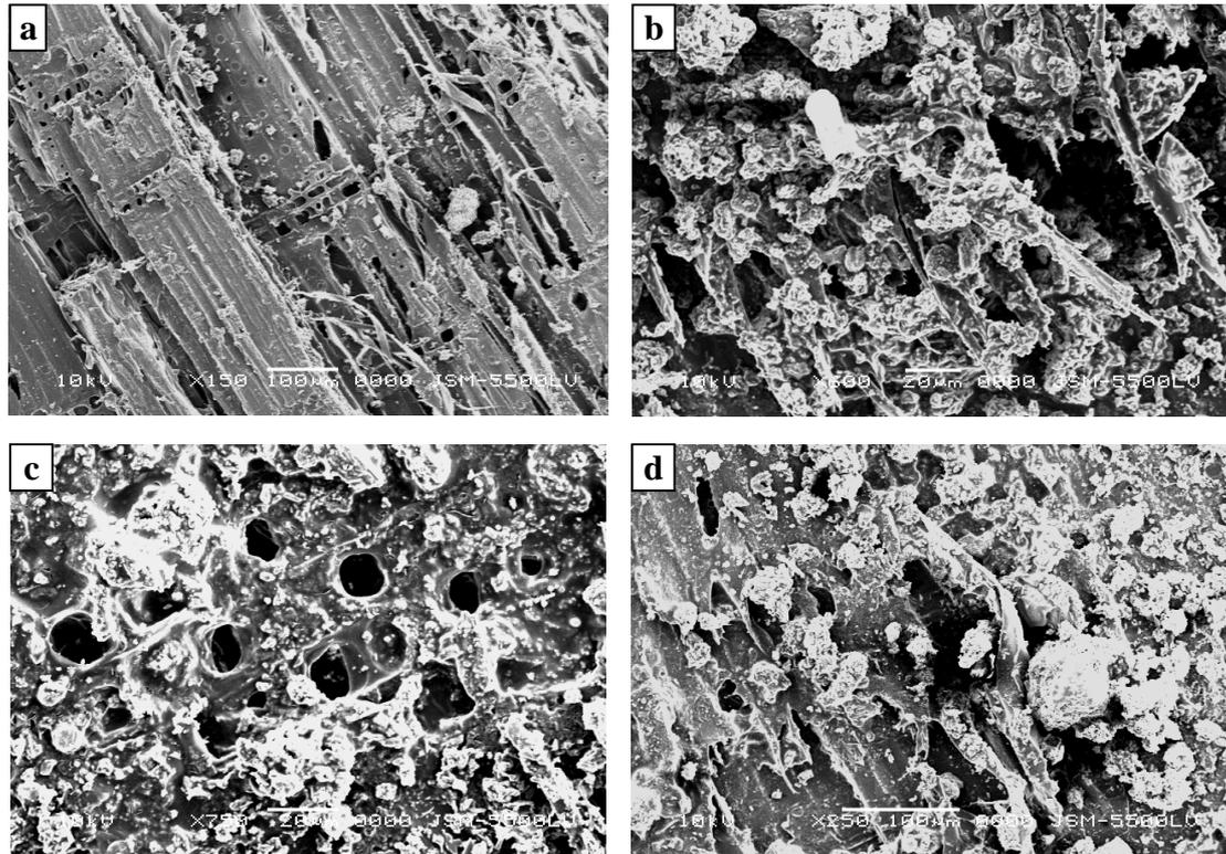
Figure (15) SEM images of the wood samples tested, shows **a** weakness and growing of microorganism on the wood surface, **b** Cellulose fibrils originating from mechanical disruption of the wood cells surface by the fungal attack, **c** degraded pit membranes were observed in the inner part, **d** crystallized dehydrate calcium sulfate was found inside
