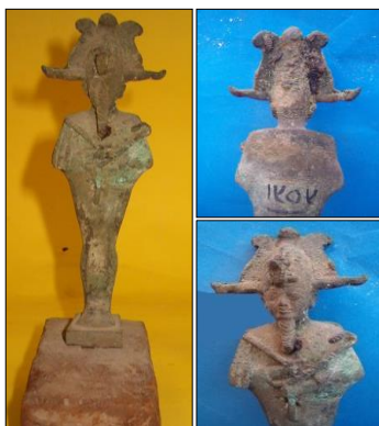
Figure (1) Shows bronze Osiris statuette, covered with corrosion layers mixed with soil.
