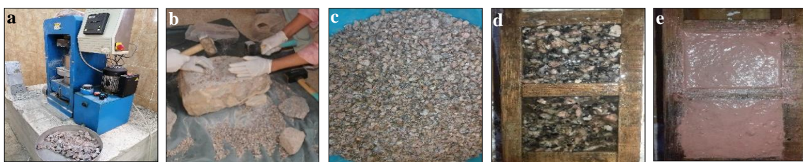
Figure (2) Shows a. & b. crushing granite by mac-hine and manually to obtain the required gain size, c. crushed granite, d. & e. preparation of cubes via pouring in a wooden mold lined with polyethylene sheets (5 cm×5 cm×5 cm)
