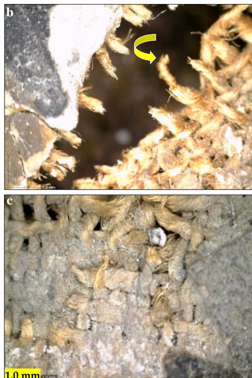
Figure (2) Shows USB microscope proves that the fibers were from linen and shows the degree of deterioration.
