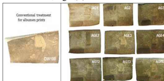
Figure (3) Shows; left sample treated with 100 % solution of distilled water, right samples post gel-based treatments and artificial aging.
