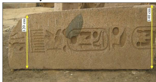
Figure (2) Shows xenolithic structure trapped in the studied granitic obelisk at Tanis.
