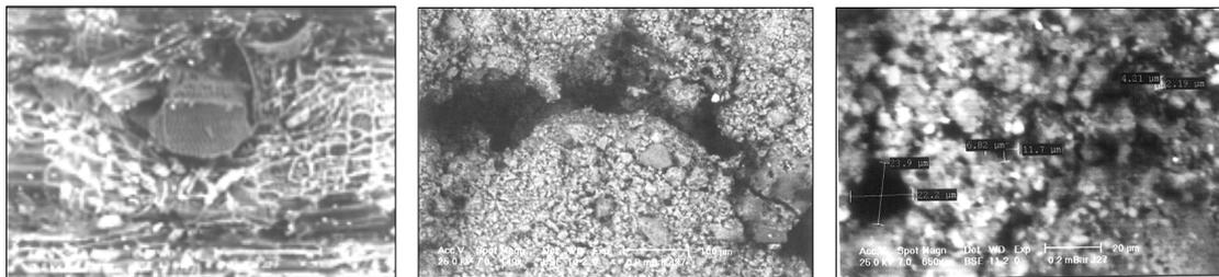
Figure (6) SEM photo of **a** friable wood structure with fungi infection chaetomium 119-182 X, **b** friable plaster and measure of grains with micronX149-650, **c** red color and measure of space between the grain with micron X250.
