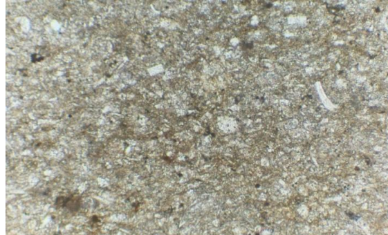
Figure (4) micro-porosity with numerous dissolute pores and microcavities in the first limestone type at Makaad Radwan
