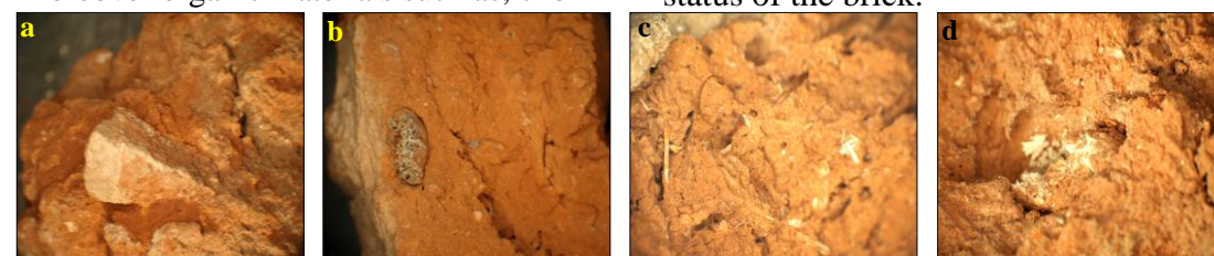
Figure (4) Shows micrographs of investigated red brick samples by LOM (4-X) a. pottery fragments, b. red brick fragment, c. different organic materials, d. animal dung.
