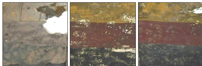
Figure (6) the wall painting models during laser cleaning compared with mechanical cleaning.
