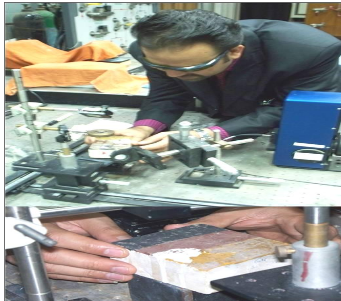
Figure (5) the wall painting models during laser cleaning, ( notice the difficulty of gypsum incrustation removing ).
