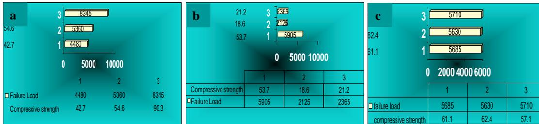
Figure (5) Compressive strength & failure load of **a. marly limestone** **b. sandy blood dolomite**, **c. white marble**
