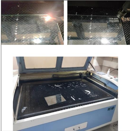
Figure (3) Shows numbering with CO<sub>2</sub> laser marker machine, (the glass mount was numbered separately, by the authors).
