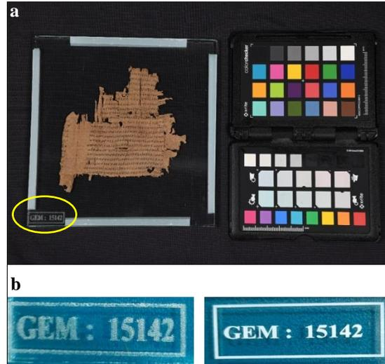
Figure (4) Shows **a.** numbering with CO<sub>2</sub> laser marker machine on glass mount; then putting the papyrus was between glass sheets, **b.** final results of numbering by CO<sub>2</sub> laser marker machine (*left*) and U.V laser printer (*right*).
