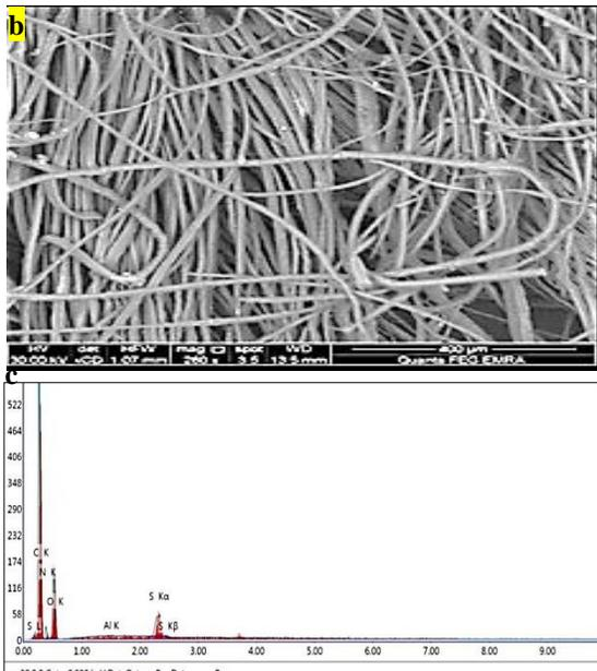
Figure (4) Shows **a.** & **b.** SEM photomicrographs results of the archaeological sample, **c.** EDX analytical results of dyed samples
