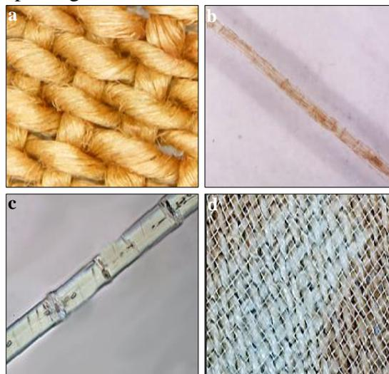
Figure (3) Shows **a.** histological structure of the artifact, **b.** historical linen fibers, **c.** linen fibers from a standard sample, **d.** dyed parts in specified areas; 10-x
