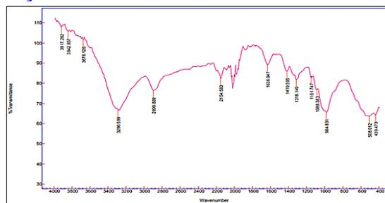
Figure (5) Shows the results of the FT-IR spectrum of a sample taken from the artifact fibers, indicating the cellulose and hemicellulose functional groups.
