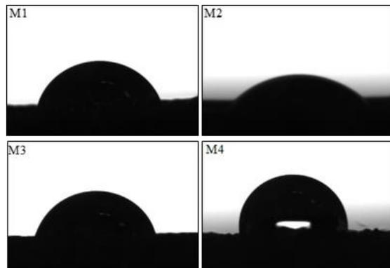
Figure (6) Static contact angle photographs of the prepared mortars.
