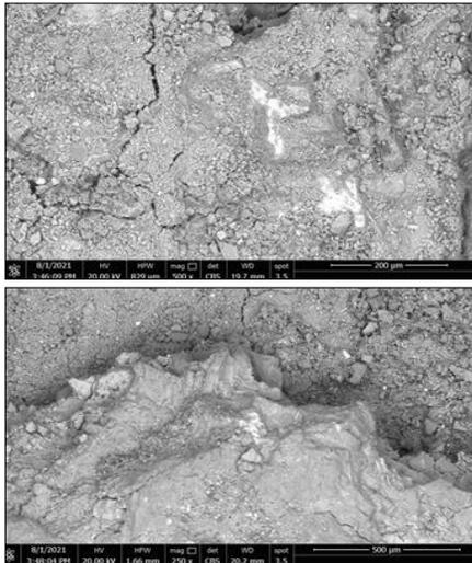
Figure (5) Shows SEM micrographs of the studied basalt surficial deformation, micro cracks, flakes and weathering products.
