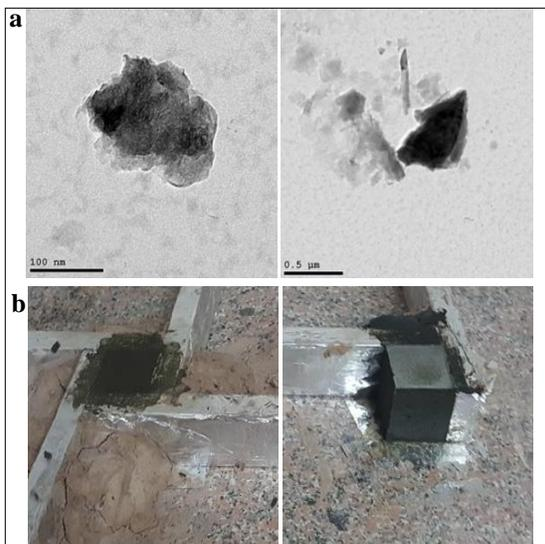
Figure (2) Shows **a.** HR-TEM micrographs of the filler material (*basaltic powder*), **b.** casting and de-moulding stages.
