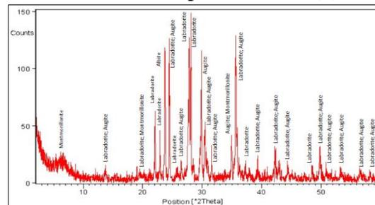
Figure (4) Shows x-ray diffraction pattern of the studied basalt.
