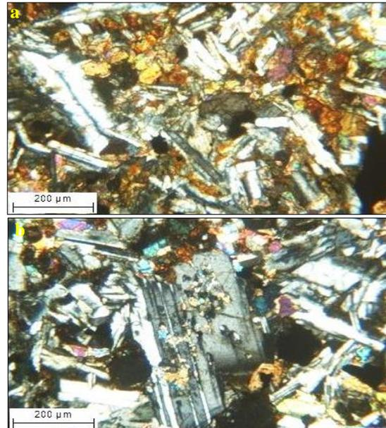
Figure (3) Shows cross-polarized micrographs of the studied basalt; **a.** phenocryst of plagioclase that altered into sericite and clay minerals and epidote, **b.** plagioclase is altered into epidote and pyroxene is altered into chlorite.
