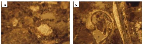
Figure (4) thin section photomicrographs of show equatorial section of nummulites Sp., clay minerals in a fine- grained matrix (biomicrite) under C.N as follow **a** 64 X, **b** 120 X
