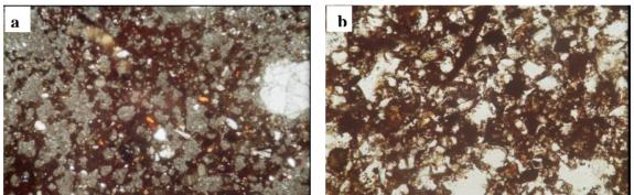
Figure (3) thin sections photomicrographs of bricks showing <u>a</u> iron oxides, clay minerals, grains of quartz and crystals of microcline and plagioclase under C.N as follow <u>a</u> 25 X, <u>b</u> 64 X
