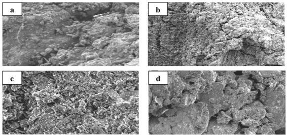
Figure (5) SEM photomicrographs showing the collapse of internal structure, voids, loose of binding material and salts crystallization between mineral grains <u>**a**</u> & <u>**b**</u> brick samples 400 X, <u>**c**</u> & <u>**d**</u> limestone samples 650 X.
