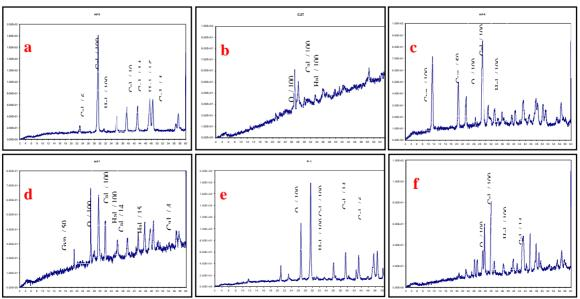
Figure (6) XRD patterns of <u>a</u> limestone, <u>b</u> brick, <u>c</u> interior plaster, <u>d</u> mortar. <u>e</u> exterior layer of plaster, <u>f</u> salts
