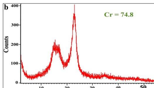
Figure (3) Shows X-Ray diffraction analysis for determination of paper crystallinity, **a.** the historical tracing paper sample, **b.** the modern tracing paper
