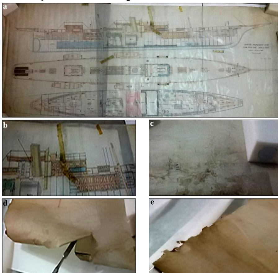
Figure (1) Aspects of deterioration of the plane; a. the screw yacht "SAFA-EL-BAHRE" plane, b. yellow pressure sensitive tape on tears, c. dirt on paper surface, d. tear in the edge, e. decay of edge.
