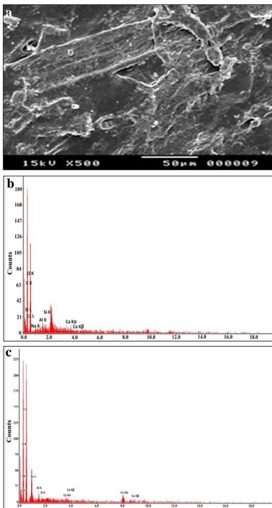
Figure (5) Shows **a.** SEM photo of the historical tracing paper sample, **b.** EDX analysis of the historical paper sample, **c.** EDX analysis of blue color
