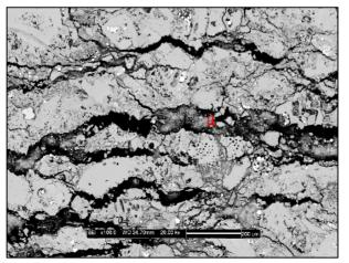
Figure (7) Shows sub-parallel stylolites and micro-cracks of the stone filled with gypsum (a).
