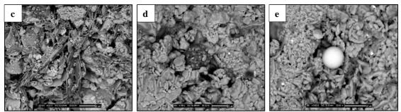
Figure (8) Shows <u>a.</u> & <u>b.</u> SEM-BSE image of surface of sample MFC3 (left) and related X-ray map distribution of sulphur (right picture), <u>c.</u> sets of platy crystals of gypsum, <u>d.</u> carbonaceous particle, <u>e.</u> smooth spherical metal particle.
