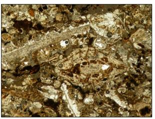
Figure (6) Shows coarse grain stone with hyaline planktonic (a) and benthic (b) calcareous foraminifera and spines of echinoderms (c) syntaxial and intragranular clear calcite cement. Nanto stone. Nicols //, 5x.
