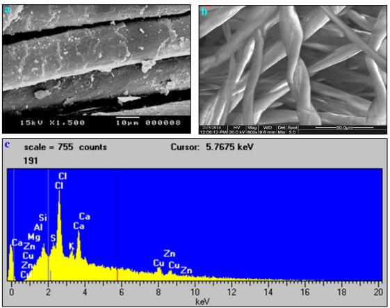
Figure (2) Shows the SEM image of the object <u>a</u>. the type of wool fiber in the strip around the textile,<u>b</u>. the body of textile is cotton, <u>c</u>. EDX chart of the dirt and stains
